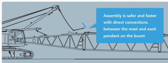
Assembly is safer and faster with direct connections between the mast and each pendant on the boom
